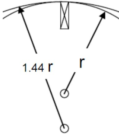
Figure 1. The two arcs of circles are shown representing the bend of floor sheathing from gravity loads. The gravity loading is assumed to be equal for both cases; however, the stiffness varies by 44 percent. The curvature is exaggerated for illustration purposes.
